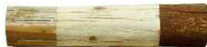
Media blasting. The bare wood shown in the middle DOES return to its natural color after media blasting.
